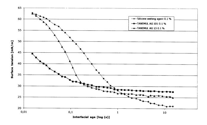
Fig.1: Dynamic surface tension measurements of TANATEX products in comparison to silicone based surfactant.
