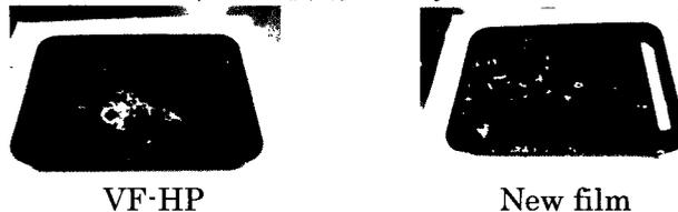
Fig. 1. Model test of spreadability for two films (2 minutes after dropping on water)
